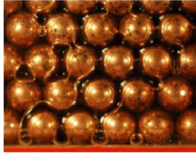
(b) Phase change process at heat flux of 37 kW/m 2
